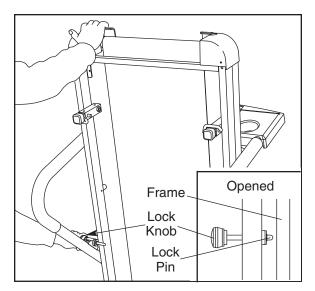
Hold the frame firmly with both hands, and lower the frame to the floor. Do not drop the frame to the floor. To decrease the possibility of injury, bend your legs and keep your back straight.
